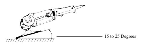
To use this tool as a sander refer to Figure 1 under ASSEMBLY directions on page four. Follow the same directions, substituting the **Sanding Disc** for the **Polishing Wheel (#46)**.
